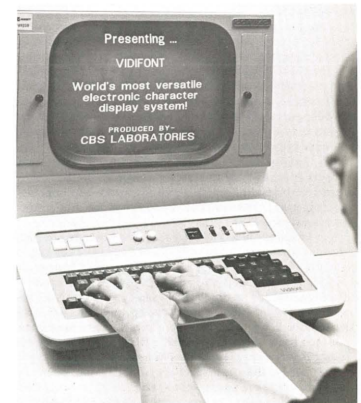
Figure 1: The Vidifont supplies characters which are compatible with superimposition.
