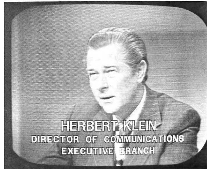
Figure 5: Character edging information is provided automatically, negating the need for additional edge generating equipment.
